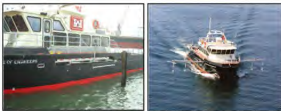
Figure 5-2. Survey Vessel Moritz Multiple Transducer Sweep System—54-ft swath with transducers spaced 6-ft c/c. Retractable boom fits flush with hull as shown in left photo. (New York District)
