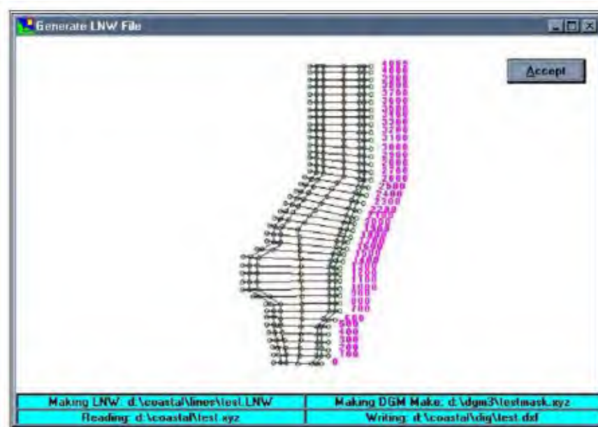
Figure 14-15. "Smart Corners" generated planned survey lines covering irregular channel alignments--cross-section alignment varies over channel intersections.
