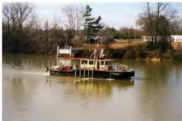
Figure 5-5. Tuscaloosa Multi-transducer sweep boats. E.B. WALLACE on left and one of three 24-ft vessels on right. (Mobile District)
