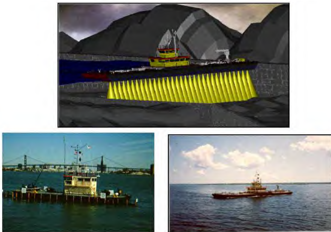
Figure 5-12. Detroit District 32-channel 120-ft sweep systems used on deep-draft navigation projects. On left, SV Bray in Detroit River (Detroit Area Office). On right, SV Bray on St. Marys River (Soo Area Office).
