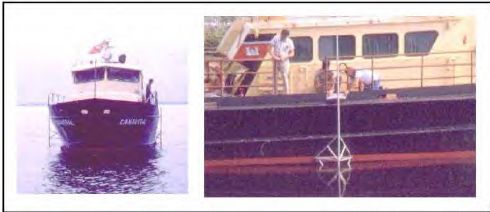
Figure 5-10. Raytheon 719 CSS three-channel hull mounted sweep ca 1970s. (Jacksonville District)
